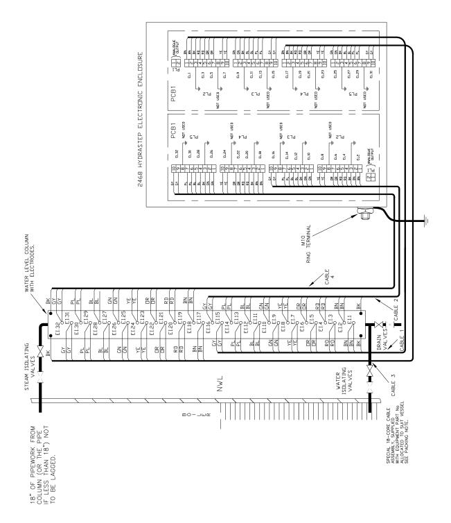
Figure 2.13 - Electrode cable connections to 32 port column
